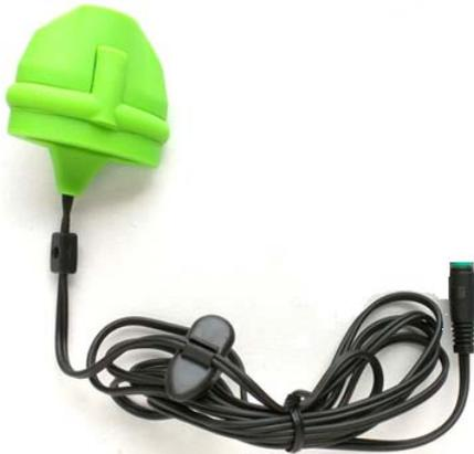
Fig. 3: Pulse Sensor
